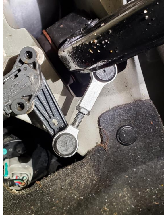
Adjustable Link Installed
