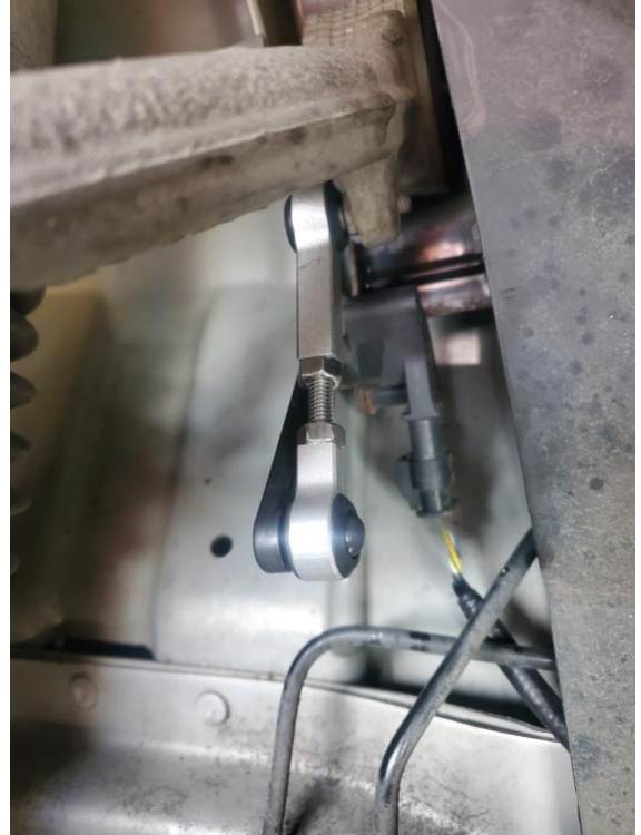
Adjustable Link Installed
