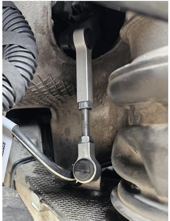
Adjustable Link Installed
