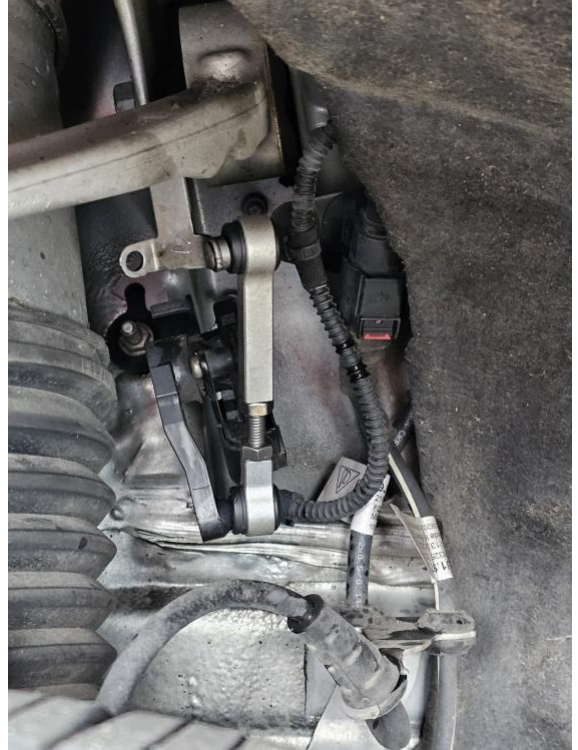
Adjustable Link Installed
