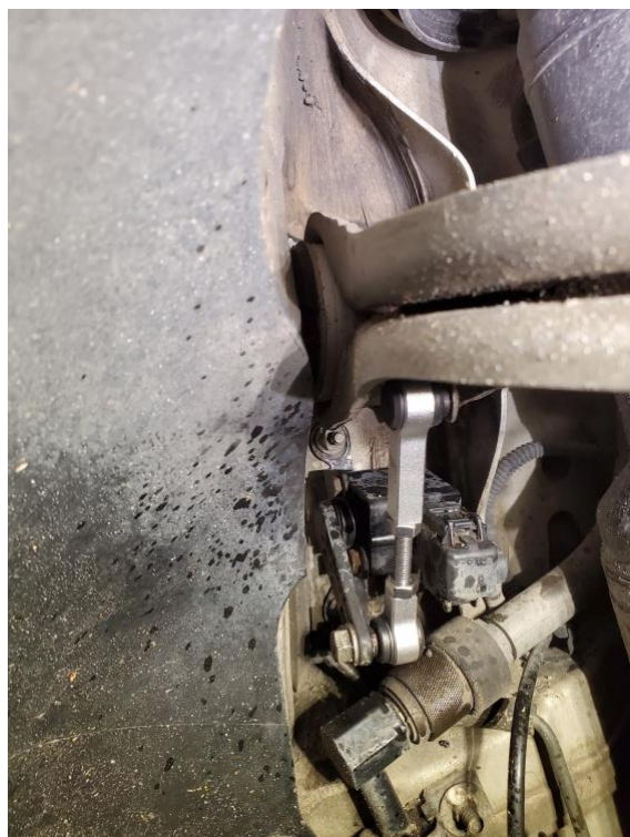
Adjustable Link Installed
