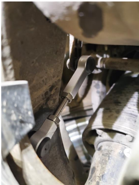
Adjustable Link Installed
