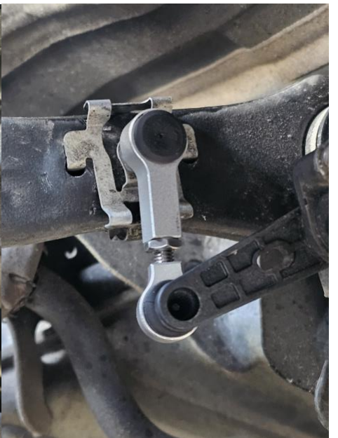
Adjustable Link Installed
