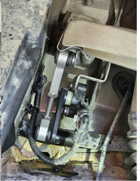
Adjustable Link Installed
