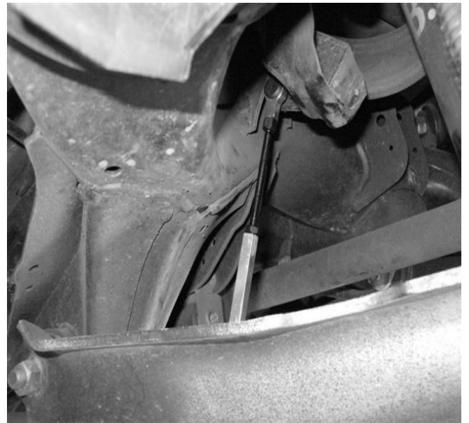
Rear Adjustable Link installed
