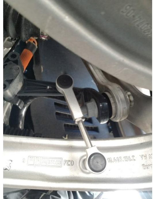
Adjustable Link Installed
