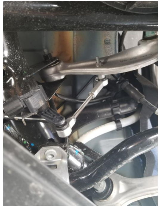
Adjustable Link Installed
