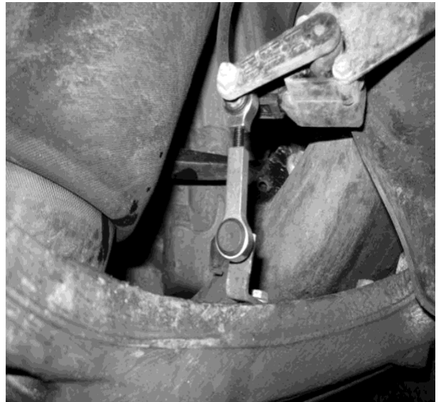
Rear Adjustable Link Installed
