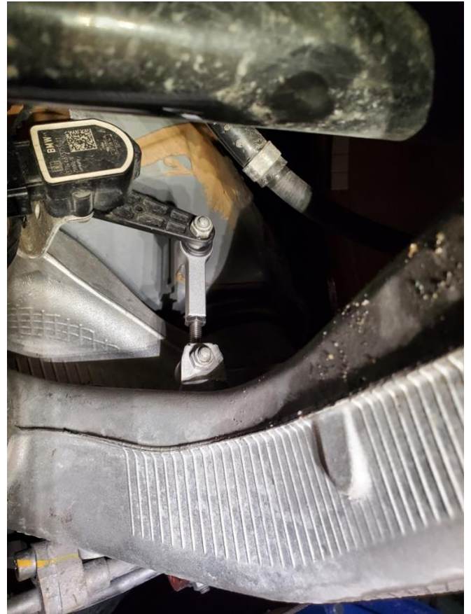
Adjustable Link Installed
