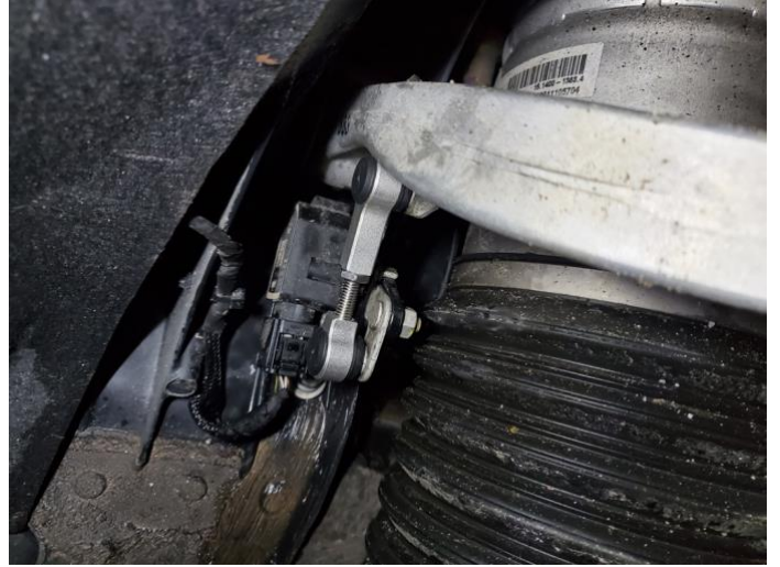
Adjustable Link Installed
