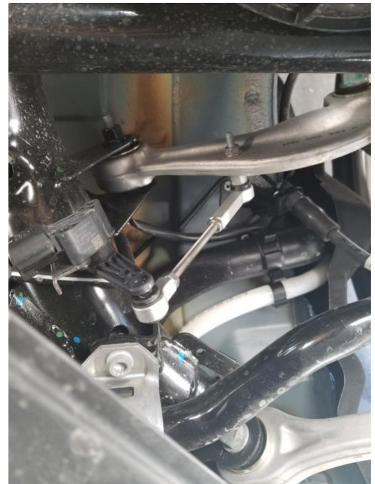
Adjustable Link Installed
