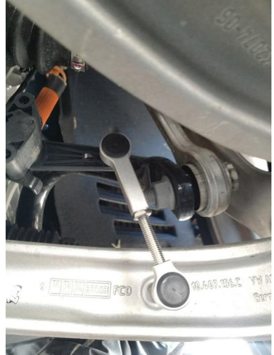
Adjustable Link Installed
