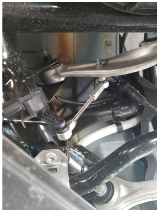
Adjustable Link Installed
