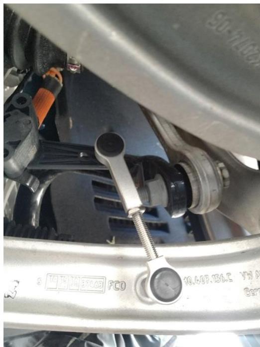
Adjustable Link Installed
