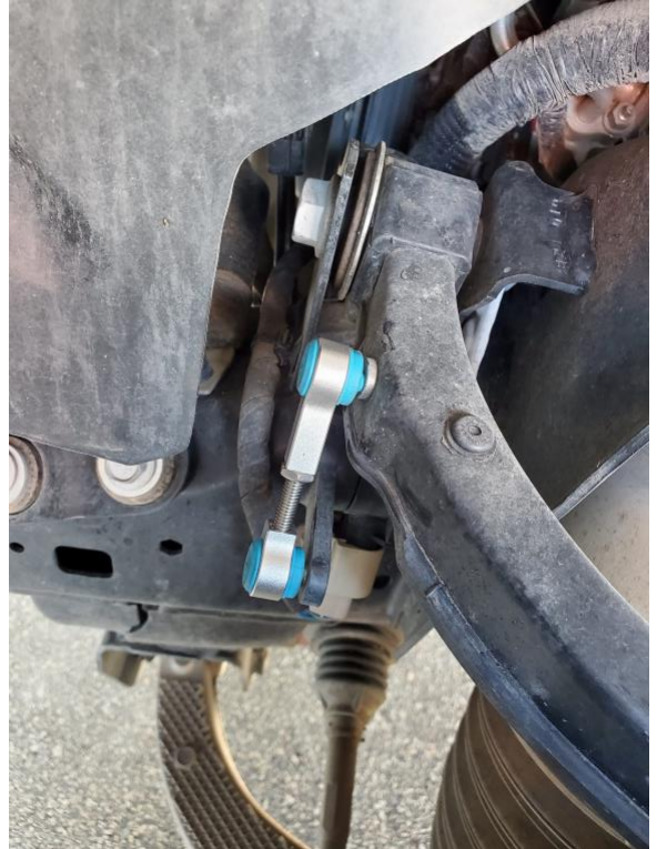
Adjustable Link Installed
