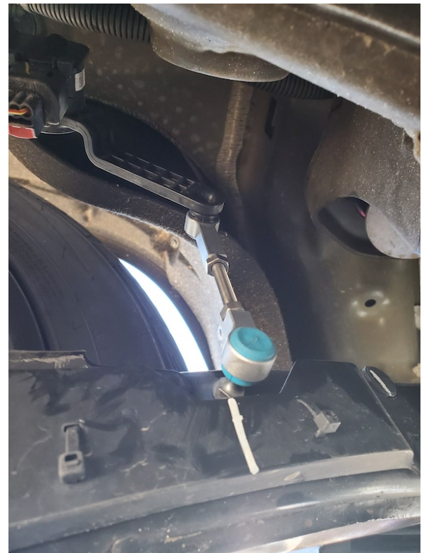
Adjustable Link Installed
