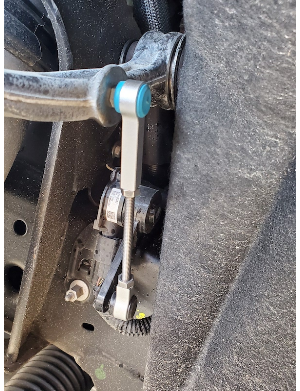
Adjustable Link Installed
