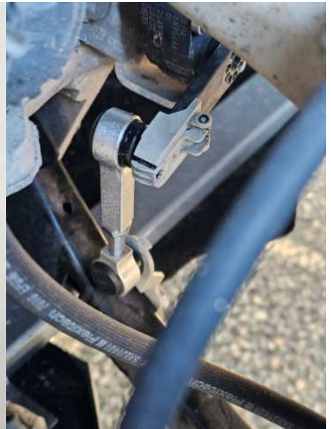
Adjustable Link Installed
