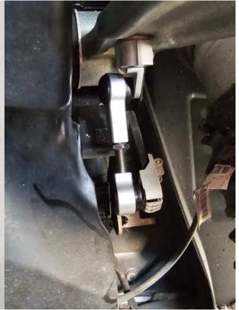
Adjustable Link Installed
