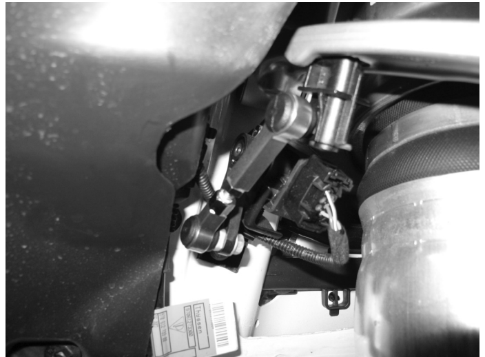
Adjustable Link installed
