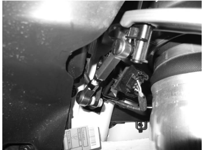
Adjustable Link installed
